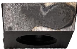
Wear on the edges of a tipped turning tool.
