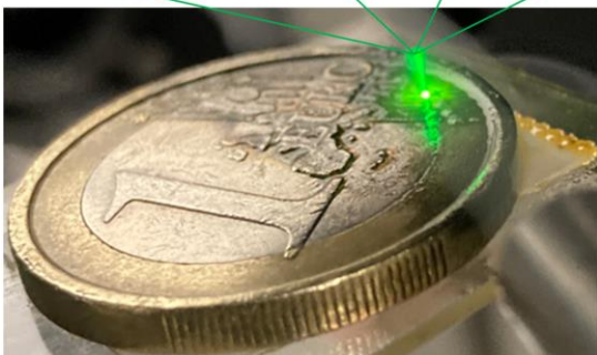
3D geometry of the star of a 1 € coin using indirect optical measurement of the surrounding fluorescent atmosphere.
