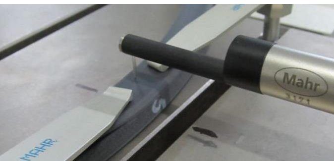
Roughness measurement on a flexible sealing element
