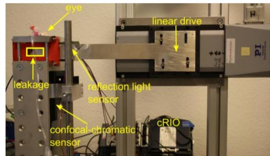
Fig. 1: Leakage test rig porcine eye on top.
