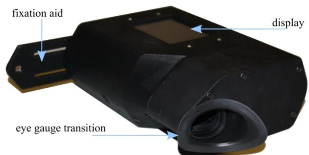
Realized self-tonometer that was used for first in vivo trials.
