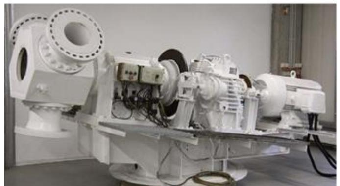
Wind turbine drive train for sensor tests
