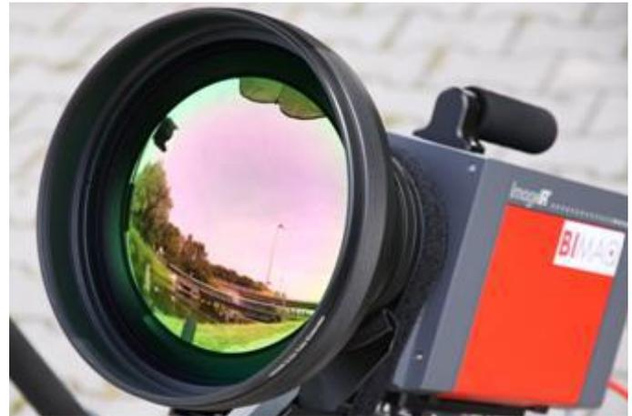
ImageIR thermographic imaging system
