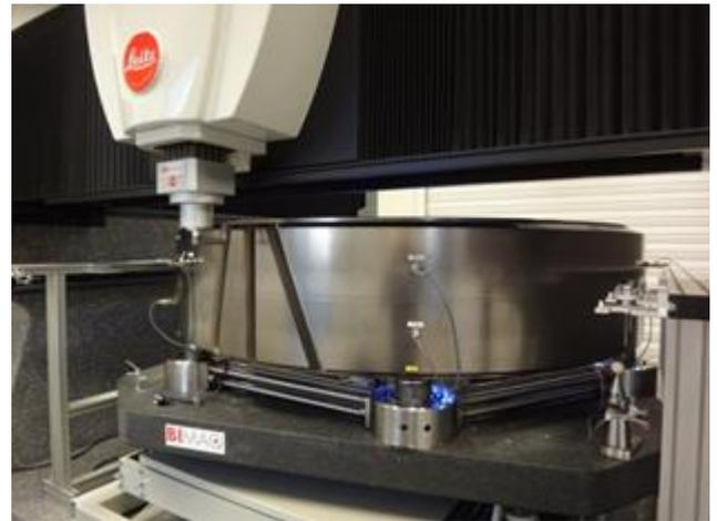
Measuring a 2 m gear standard
