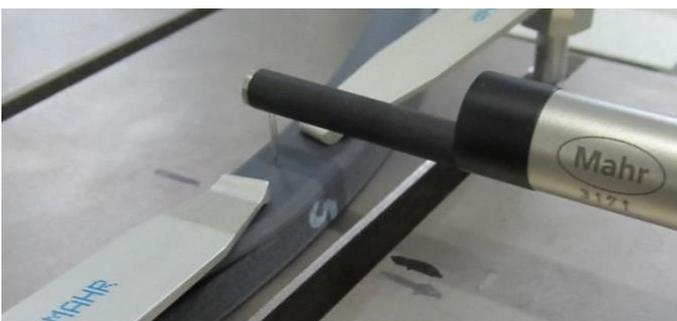
Roughness measurement on a flexible sealing element
