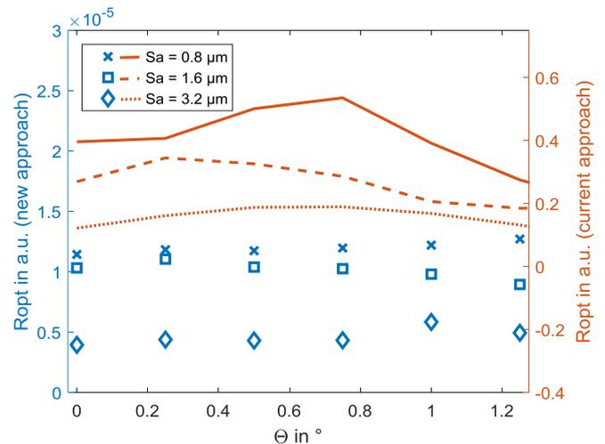
Result of the current (orange) and the newly proposed (blue) speckle evaluation algorithm with integrated surface tilt correction over the tilt angle  $\Theta$ . Note the different axis scaling of  $R_{opt}$ , which is the output quantity of the measurement system that corresponds with the surface roughness. As a result, the cross-sensitivity with respect to the surface tilt angle is eliminated.
