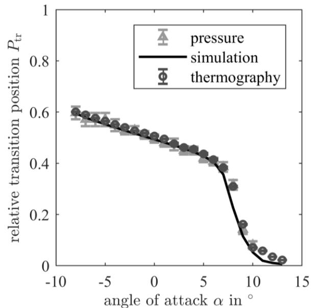
Relative position  $P_{tr}$  of the laminar-turbulent transition
