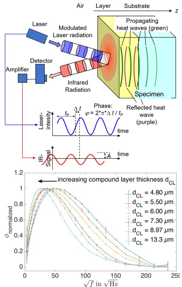
Top: Principle of photothermal radiometry.
