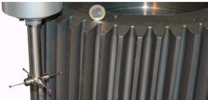
Tactile measurement of large cylindrical gearing
