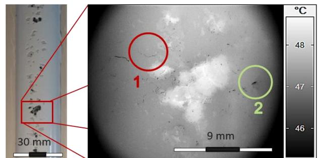
Thermogram of an eroded test sample; 1: micro-crack; 2: subsurface material inhomogeneity.
