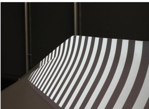
Reference measurement on a blade by means of stripe pattern projection.
