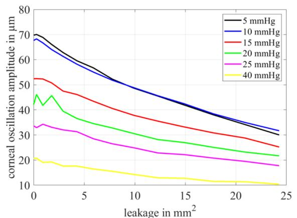
Fig. 2: Corneal deflection according to leakage at six IOP values.
